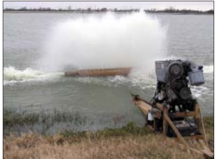
Figure 17. Pump-sprayer or "bankwasher" type diesel aerator.
