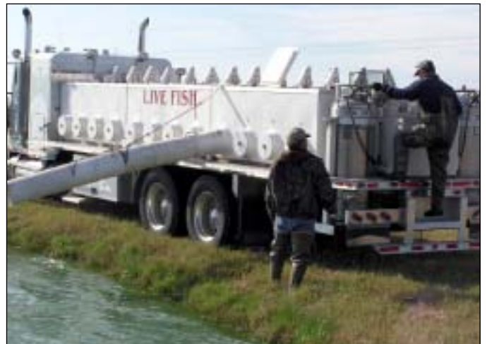
Figure 24. A live-haul truck for transporting fingerlings and food fish.
