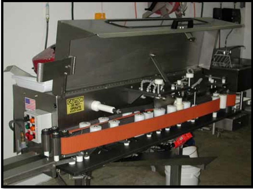
Fish filleting machine (above)
