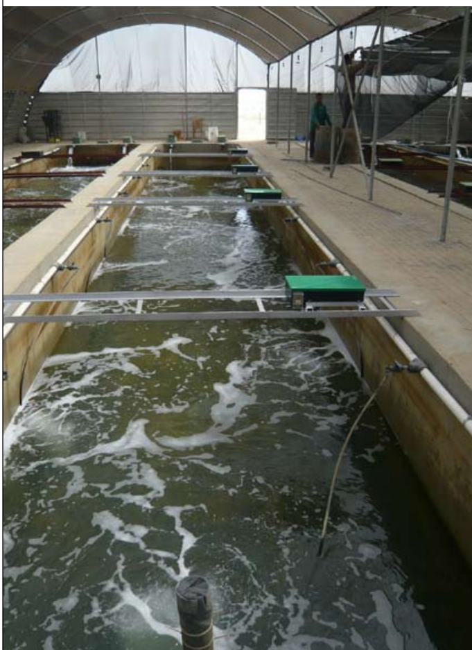
FIGURE 12 European seabass nursery raceway tanks (100 m 3 ) with air-diffusers in Rula land reclamation company, Wadi Group, El-Beheira Governorate, Egypt
