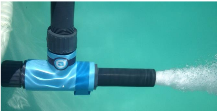
Figure. Solids removal device used in the biofloc juvenile shrimp raceways at Bowers Shrimp
